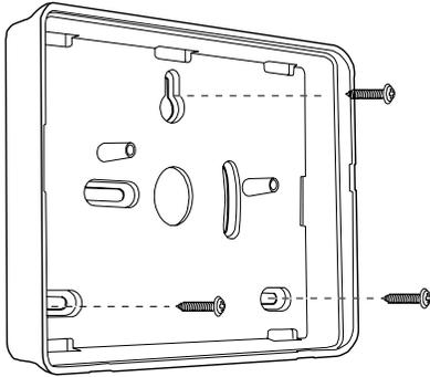
Figure 11 Screw Keypad Back Box to Wall
