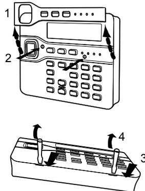
Figure 6 Opening the Keypad
