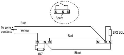
Figure 19 Example: Wiring Two Door Contacts to One FSL Zone.
