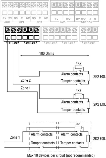
Figure 18 Fully Supervised Loop Zone Wiring
