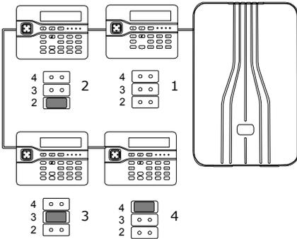
Figure 14 Keypad Addressing Jumpers
