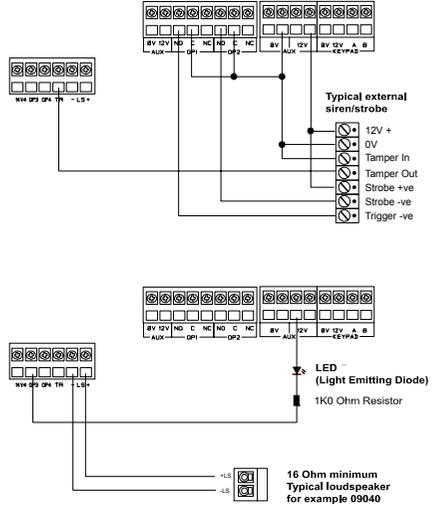
Figure 20 Connecting Wired Peripherals
