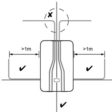
Figure 15 Mains Cabling Clearance
