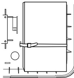
Figure 22 Fitting the Battery
