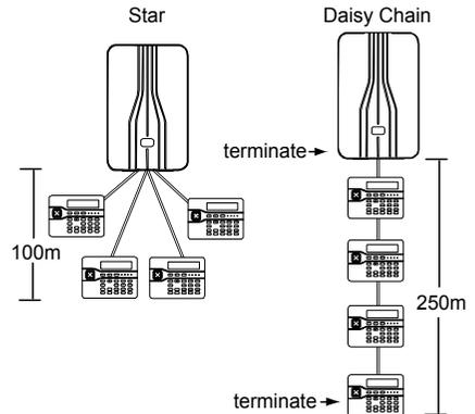
Figure 12 Keypad Wiring Configurations
