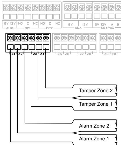
Figure 17 Closed Circuit Loop Zone Wiring
