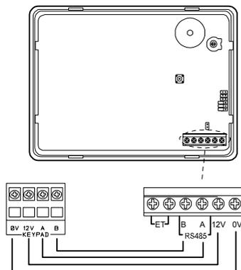
Figure 13 Keypad Connection
