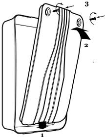
Figure 23 Replacing the control unit lid.
