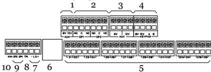
Figure 4 Control Unit Main Connectors
